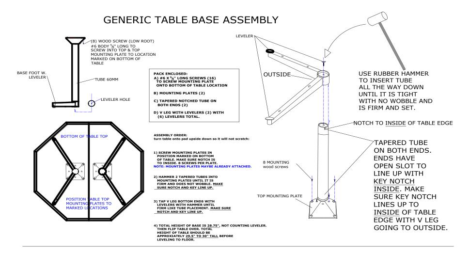
CAUTION: PLACE TABLE TOP UPSIDE DOWN ON PAD OR PROTECTIVE COVER BEFORE HITTING POST COLUMNS INTO MOUNTING PLATE. TAPER IS DESIGNED TO FIT TIGHT
